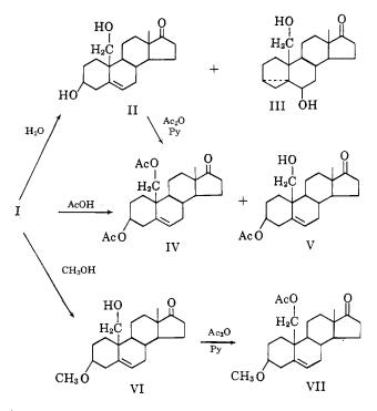
The nature of the *p*-toluenesulfonate was not determined but it is presumably  $3\beta$ -*p*-toluenesulfonoxy-19hydroxyandrost-5-en-17-one. Further experiments are planned for the isolation and characterization of this product.
